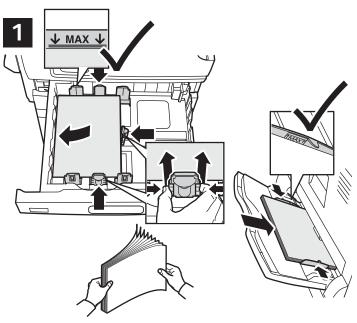
For the best results, fan the edges of the paper. Adjust the guides to fit the paper size. Do not load paper above the maximum fill line.
