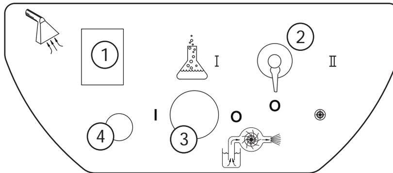
**Vacuum Switch (1):** turns on the vacuum motor.
